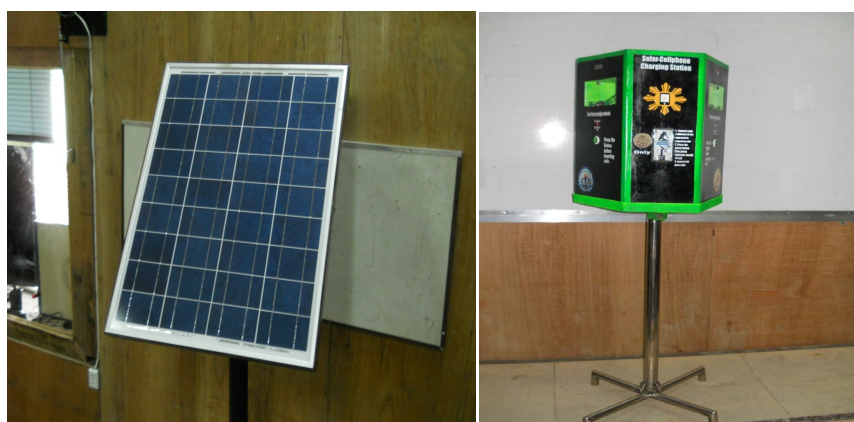
Figure 2. Solar module for powering the system and the solar powered cell phone charging station.
