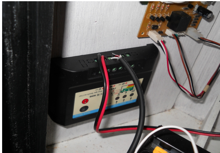
Figure 4. Solar cell control module and regulator circuit.
