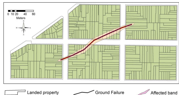
Figure 4. Cartographic inputs: property (polygon), aseismic ground failure (line) and influence band (polygon).
