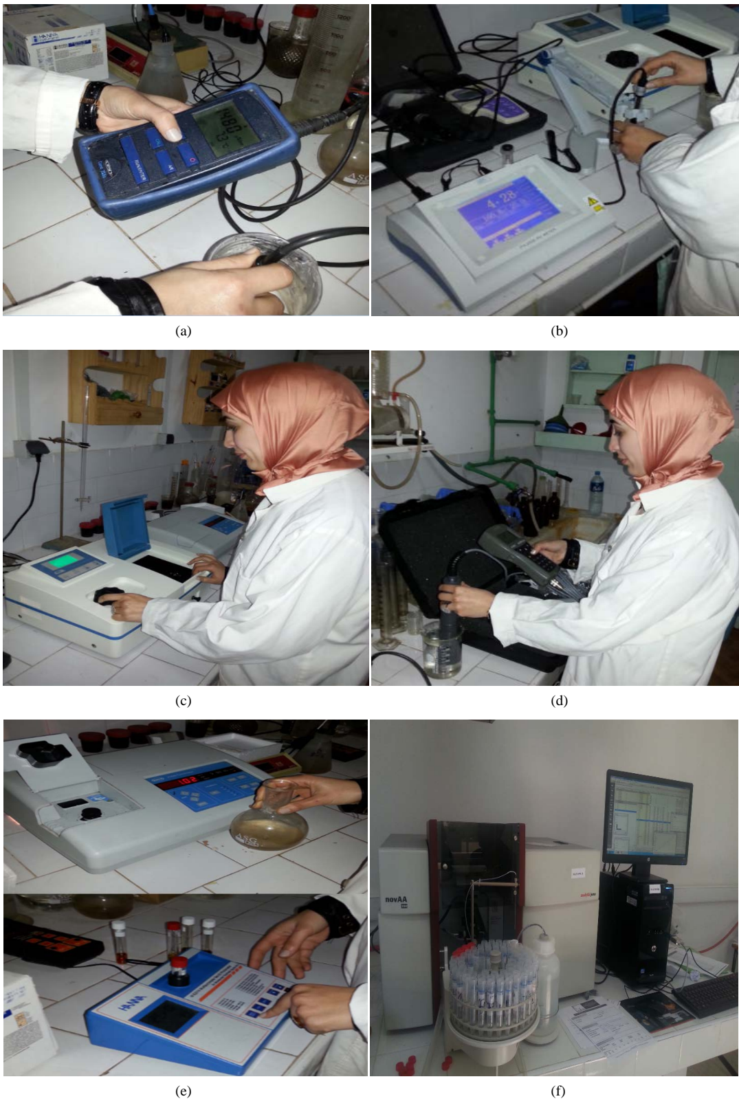
Figure 5. Methods of analyses of raw water in Laboratory of Environment (Faculty of Science Kenitra). (a) Conductimeter; (b) pH meter; (c) Spectrophotometer; (d) Multiparameter; (e) Turbidimeter and multiparameter; (f) Atomic absorption spectrometry.
