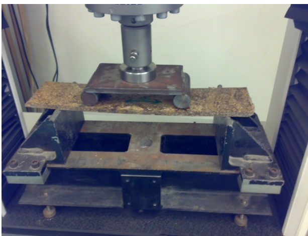
Figure 2. The flexural fixture with 3 point bending.
