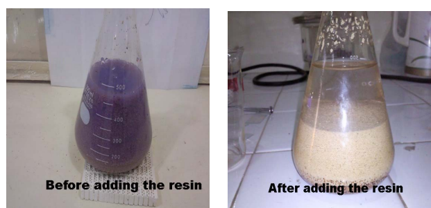
Figure 1. Photo shows ion exchanging before and after adding the clean resin to the solution of cesium and cobalt.
