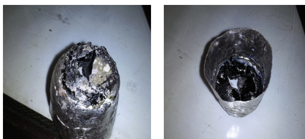
Figure 11. Photos show the damage in the upper and lower parts of a platinum crucible due to sulfur reaction under air atmosphere.
