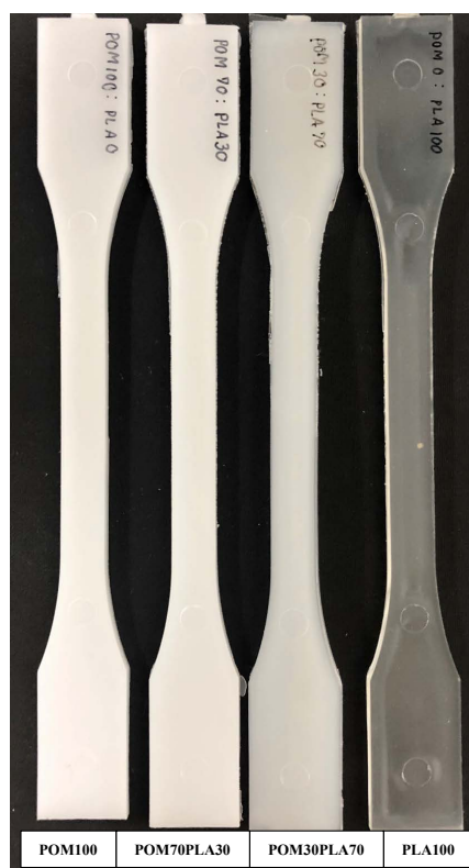
Figure 1. Photographs of dumbbell shaped specimens of POM, PLA, and their blends.
