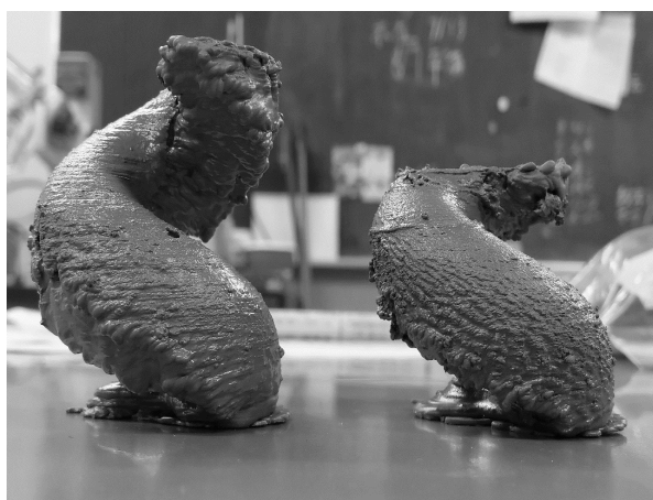
Figure 10. Appearance of the molded bodies with 20% reduced hollow spiral shape using the composition. No. 7 (diluted by water) and No. 16 (water + nanosilica).
