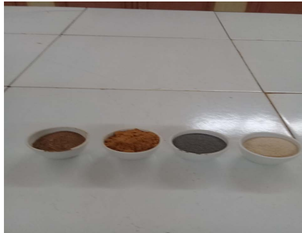
Figure 1. Ashes samples for BLA LBPA, GSA and RHA after calcinations.
