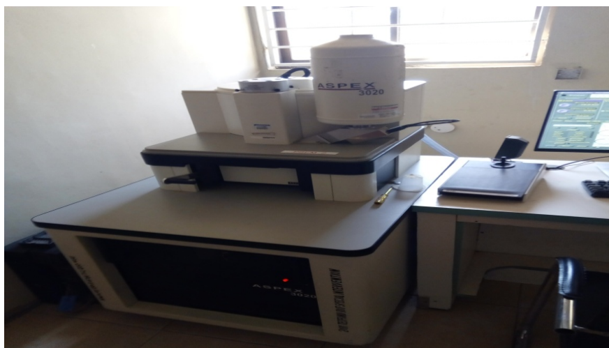
Figure 2. Scanning electron microscope used for the research.
