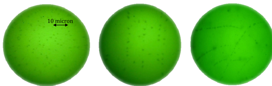
Figure 1. State of clusters of Ni atoms in silicon. (a) After diffusion; (b) After thermal annealing at T = 850^\circ\text{C} ; (c) After thermal annealing at T = 650^\circ\text{C} .
