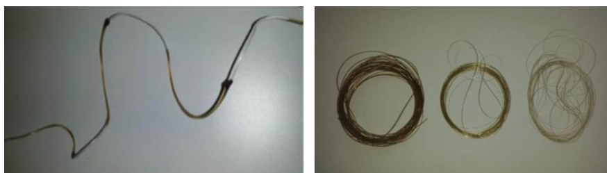
Figure 7. PP-based core-sheath fiber with partially torn sheath due to incompatible parameters (left); homogeneous PP-based core-sheath fibers possessing different draft rates, from left to right 1:1, 1:4 and 1:8 (right).
