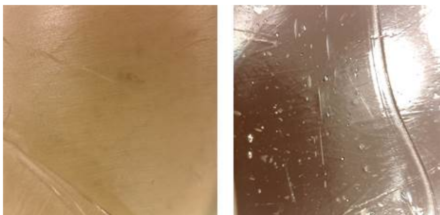
Figure 5. Microscopic view (correspond to 7 \times 7 \text{ mm}^2 ) of the produced composites from the synthesized magnetic core-shell nanoparticles in PP (left) and PA 6 (right).
