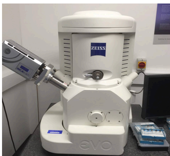
Figure 5. Scanning electron microscope couple with energy X-ray dispersive analyser (SEM/EDAX) (the Zeiss EVO LS10) instrument.
