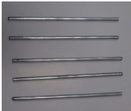
Figure 2. Hot dipped steel reinforcements used in this study.
