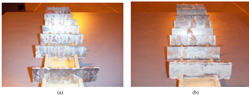
Figure 12. Chromium plated samples photographed after (a) 24 Hours and (b) 96 hours in a CASS testing chamber.
