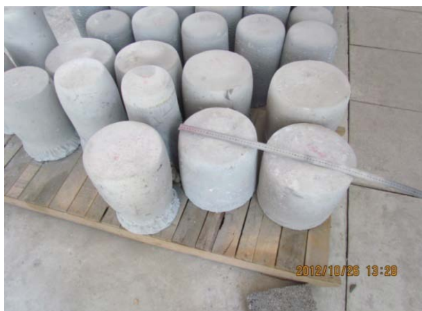
Figure 1. Billets of Al alloy by spray forming.
