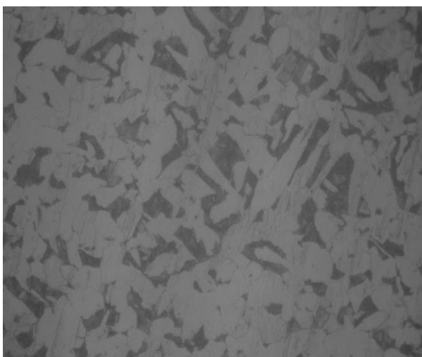
Figure 1. Microstructure of API5L X52 base metal (4'' pipeline material).
