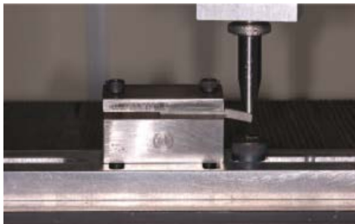
Figure 2. Cast bar and secured in a vise with the application load testing machine (bar deformed by the action of the force).
