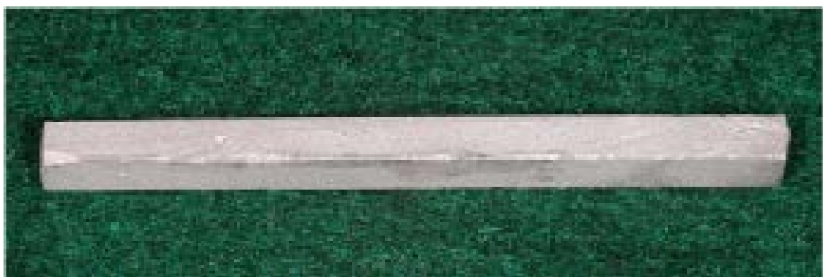
Figure 1. Complete bar to be subjected to compressive loading (experimental sample).
