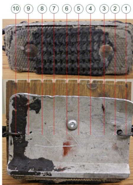
Figure 5. Load application location on the ladder shoe for friction tests.
