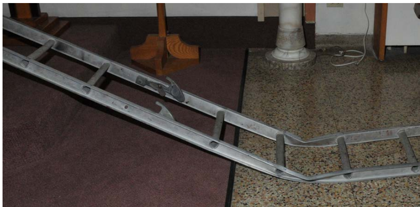
Figure 4. Portable ladder buckling.
