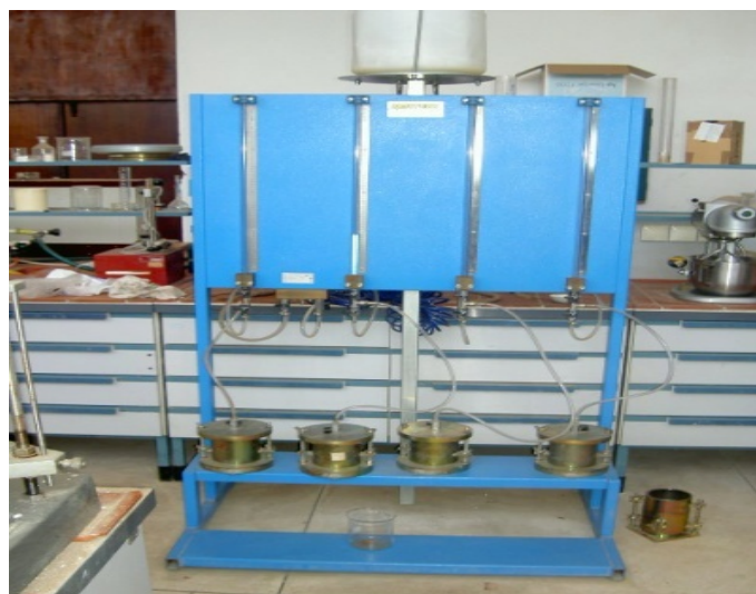
Figure 8. Photography of the device of the permeability test with a permeameter of compaction.
