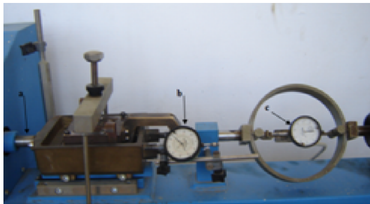
Figure 11. The UU shear test device.
