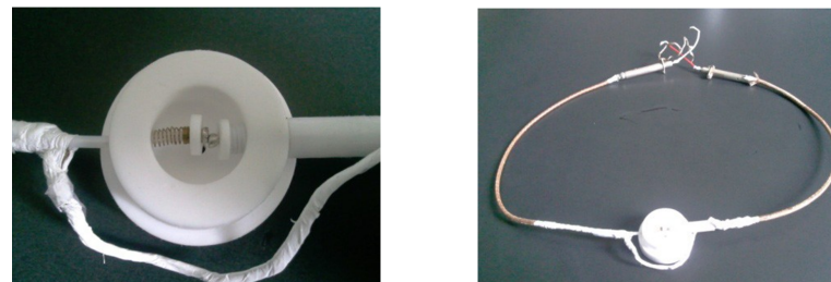
Figure 4. The Teflon chamber is connected to the NPDI with its coaxial cables.
