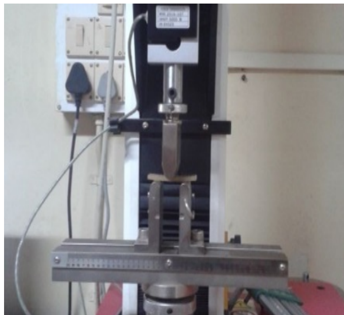
Figure 6. Horizontal shear load diagram and test setup ILSS test.
