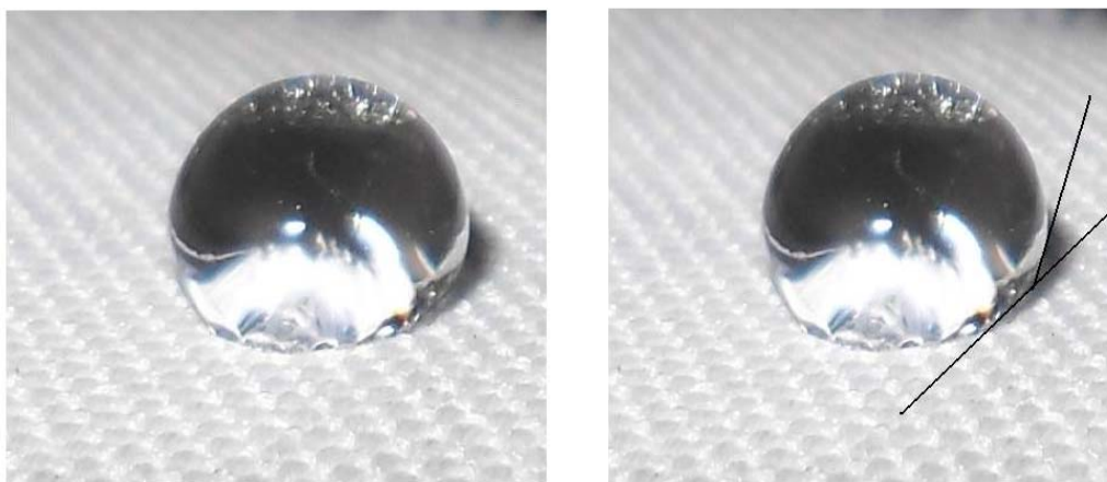
Figure 2. Water drop photo of plasma- \text{Al}_2\text{O}_3 treated PET at 1.3 watt for 2 min.
