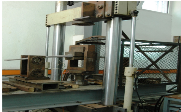
Figure 1. The test rig in the AISI 6150 steel leaf spring static fatigue tests [14].
