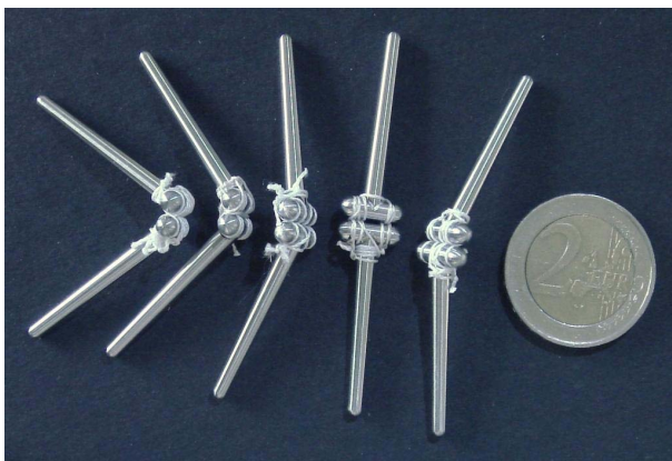
Figure 15. Set of fiber-hinges with one degree of freedom; rotation around one axis. The size as compared to a 2 Euro coin illustrates the possibility of design as a potential finger joint implant.
