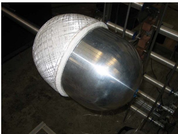
Figure 9. Preform with "fiber weld" at the cutting location.
