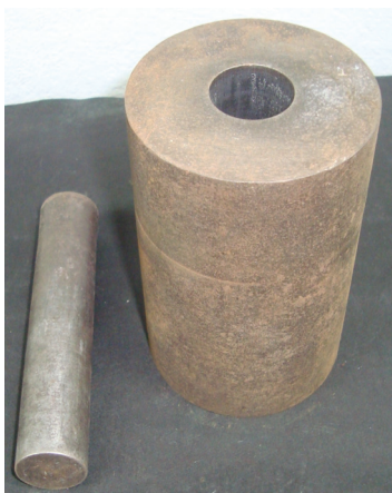
Figure 4. Metallic die with punch.
