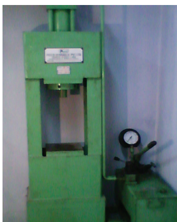
Figure3. Manual type hydraulic press.
