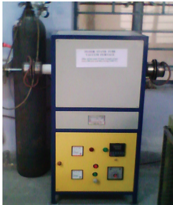
Figure 5. Induction type floor stand tube vacuum furnace.
