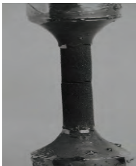
Figure 11. An illustration of catastrophic crack formation in a stress corrosion specimen after failure in 52 Wt% NH 4 NO 3 solutions of pH 9.64 at 368° K.
