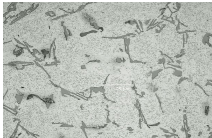
Figure 5. Microstructure of 6 wt.% composite cast using copper chill of 25 mm thickness.
