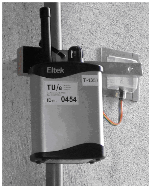
Figure 4. Measurement of the surface temperature and relative humidity using a box.
