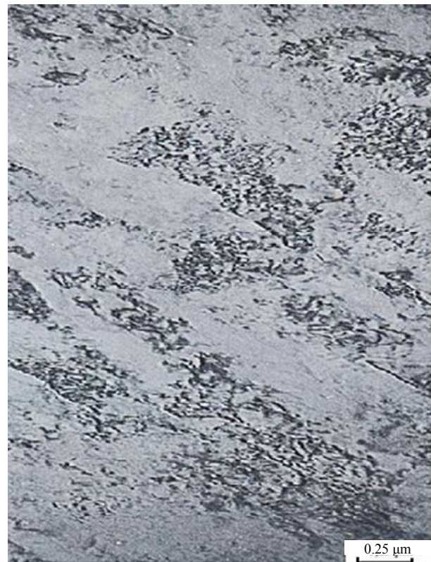
Figure 3. Development of slide bands ( t = 3.6 ks).
