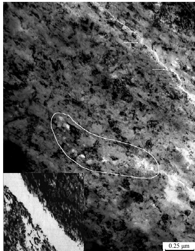
Figure 2. Development of microcracks (arrows) ( t = 0.9 ks), the inset ( t = 5.4 ks).
