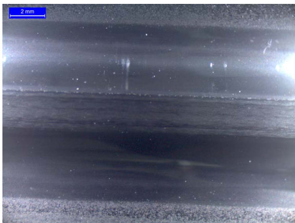
Figure 10. Light wear on the inner raceways with polishing of the contact zone (test 1).
