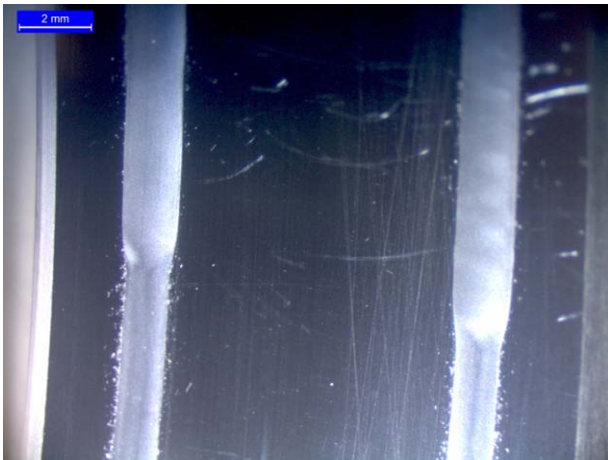
Figure 8. Heavy abrasion with a noticeable different deformation at the point of entering the contact zone (test 1).
