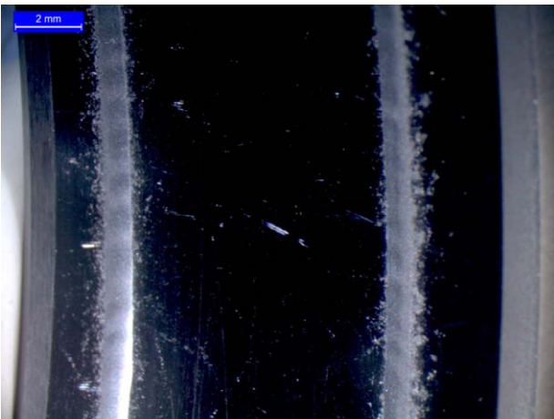
Figure 9. Abrasion of the outer ring raceway with a wave like deformation of the raceways (test 2).
