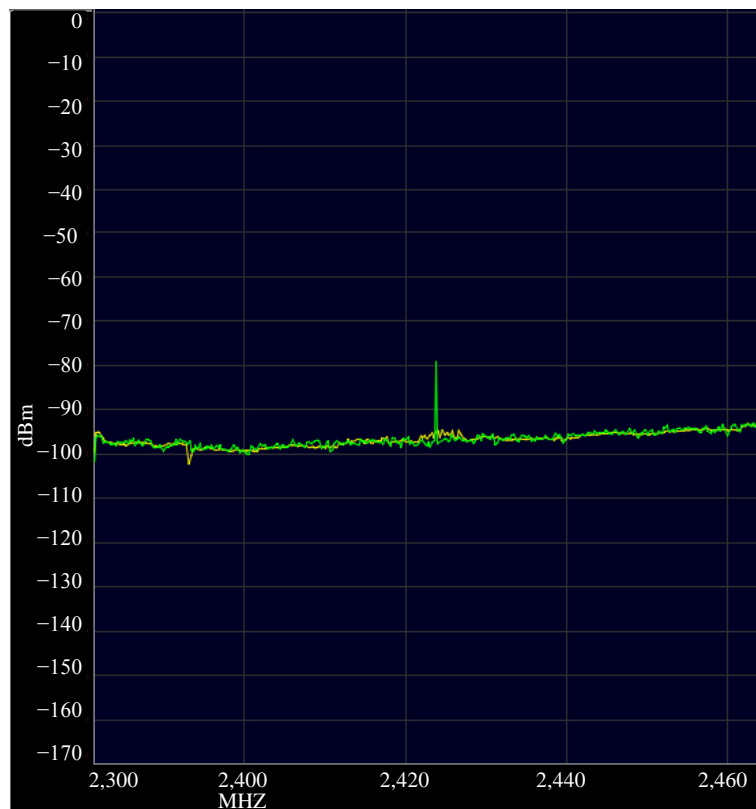
Figure 7. A detected signal from a test 2.5 GHz source in air at a 0.25 m distance.
