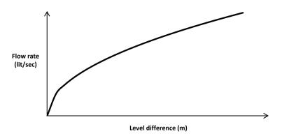
**Figure 3.** Variation of flow rate with level difference between filter and over flow tank.
