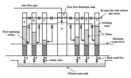
Figure 2. Schematic layout of the overflow controlled declining rate filter model.
