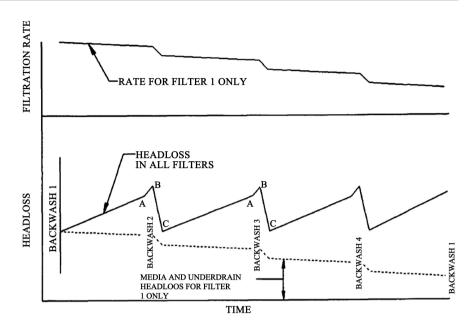
Figure 1. Filtration rate and head loss during one filter run in declining rate filters [14].
