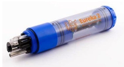
Figure 4. Data logger: Eureka Manta2™ used for in situ monitoring.
