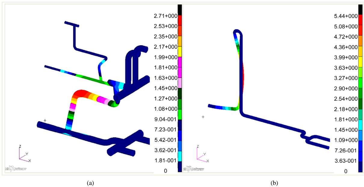
Figure 9. Frequency response analysis of fluid and air pipes during the backwash. (a) 1st mode of water pipe, 13.33 Hz; (b) 1st mode of air pipe, 22.69 Hz.
