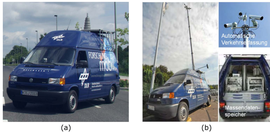
Figure 8. (a) The DLR UTRaCar with retracted telescopic mast. (b) The DLR UTRaCar with extracted telescopic mast [14].
