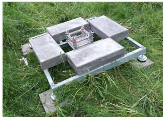
Figure 12. The ground base of the portable pole is equipped with tiles, adjustable feet, and a swivel bracket to ease the raising of the lattice mast.
