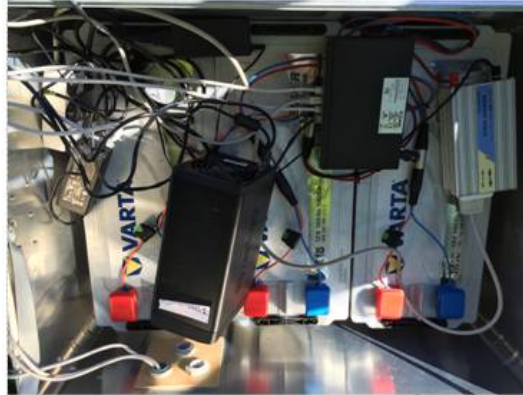
Figure 3. The Eurobox 40705 containing 3 batteries, a 230 V power inverter, a PoE switch, and a NAS server.
