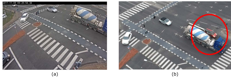
Figure 1. Objects can overlap each other in the camera-view as seen in (a) where the large concrete truck clearly occludes the lane behind it. (b) Clearly shows that a red car is in fact driving side-by-side of the concrete truck.
