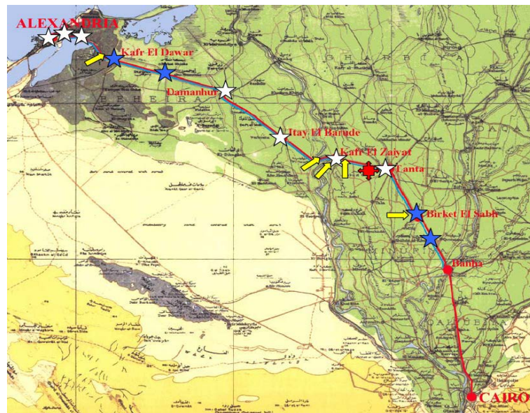
Figure 2. The Cairo-Alexandria railway line (red line) and the Arab El Raml-Alexandria signaling system upgrading sector (blue line), showing the approximate locations of existing dispatcher towers (☆), proposed dispatcher towers (★), draw bridges (◆) and the Tanta traffic control center.
