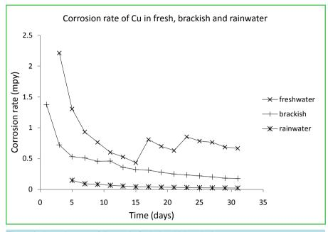
Figure 2. Corrosion rate of Copper in fresh, brackish and rainwater.
