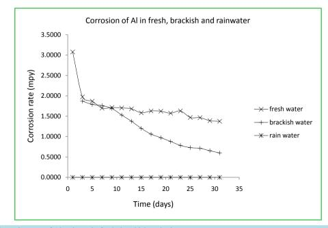
Figure 1. Corrosion rate of Aluminum in fresh, brackish and rainwater.
