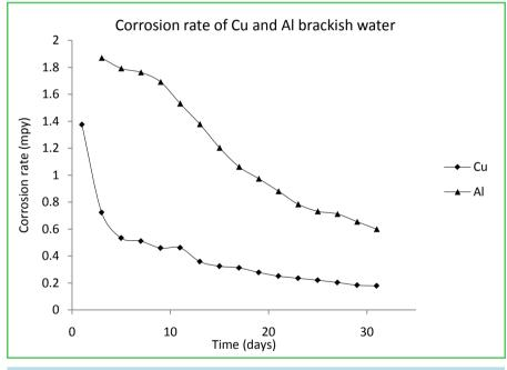
Figure 3. Comparison between rate of corrosion of copper and aluminum in brackish water.
