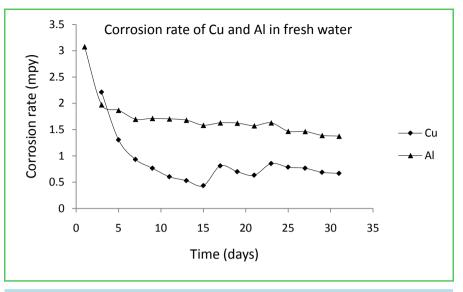
Figure 4. Comparison between rate of corrosion of copper and aluminum in freshwater.
