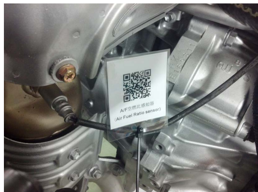
Figure 2. QR code is labeled on sensor.
