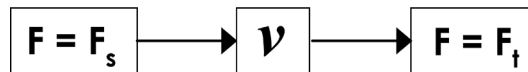
Figure 3. Effect of target speed ( v ) and measurement system stability. Transduction of magnetic signal F = F_s (static signal) by means of measurement action ( F = F_t \rightarrow transient signal). Observed field F = F_{(s,t)} .
