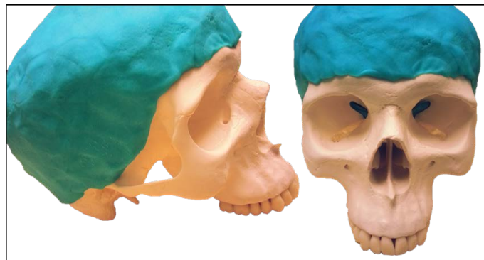
Figure 1. Synthetic three-shell realistic head model consisting of electroconductive dough which lines the inner and outer surfaces of a replica human skull. Lateral (left), rostral (right) views of the model showing the scalp layer.
