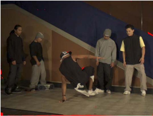
Figure 8. Refinement of initial synthesized image (image in Figure 7) by using graph cut (the red color pixels are disoccluded pixels).
