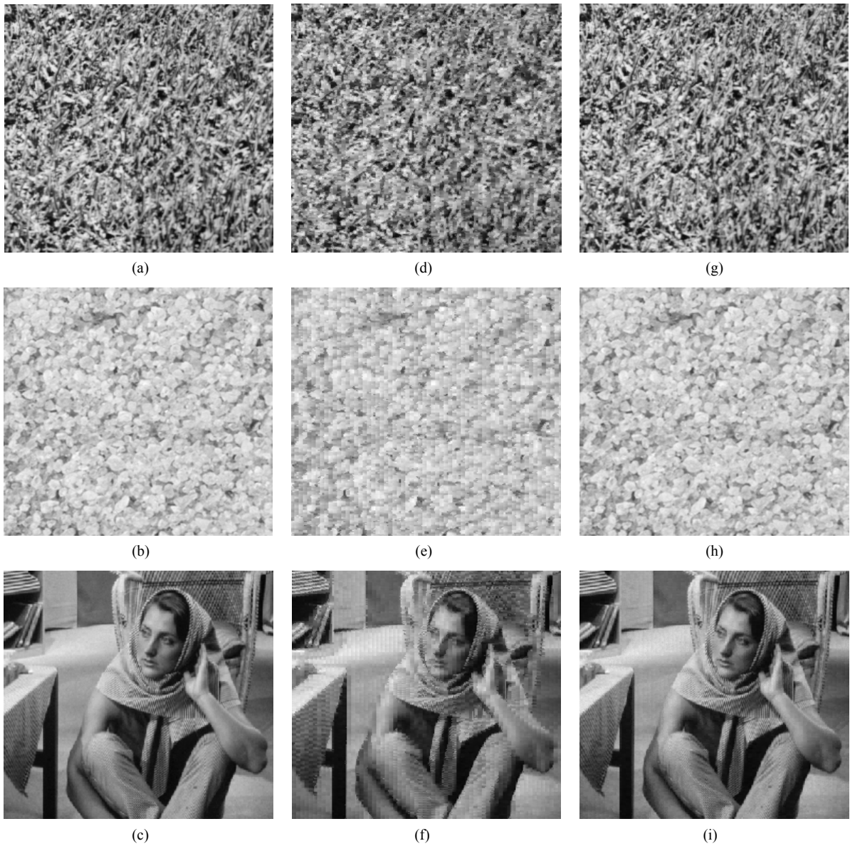
Figure 4. (a), (b) and (c) are original images; (d), (e) and (f) are reconstructed images by the proposed model; (g), (h) and (i) are reconstructed images by JPEG with quality factor 60.
