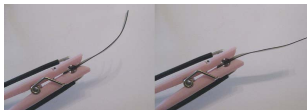
Figure 2. Activation of IPMC film. Supplied by Environmental Robots Inc.
