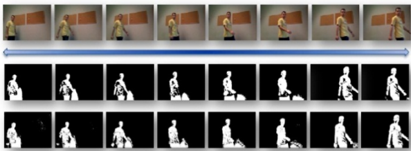
Figure 3. Execution of “running average (RA)” (second row) and “Gaussian mixture model (GMM)” (third row).
