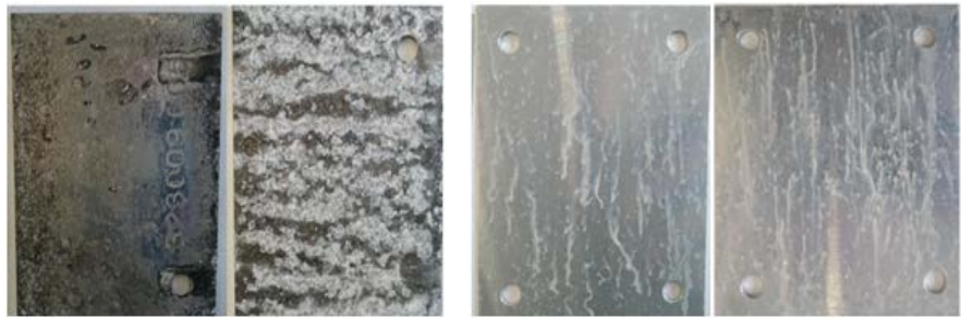
Figure 4. Result of untreated and treated AA7075 alloy with various coating mass ( 0.16 \text{ g/m}^2 ) left and ( 0.36 \text{ g/m}^2 ) right.
