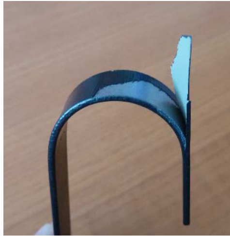
Figure 4. Sample number 21 (TC + PL). Chipped base + topcoat + plasma. Sample bent on a graduated bending jig with rollers.
