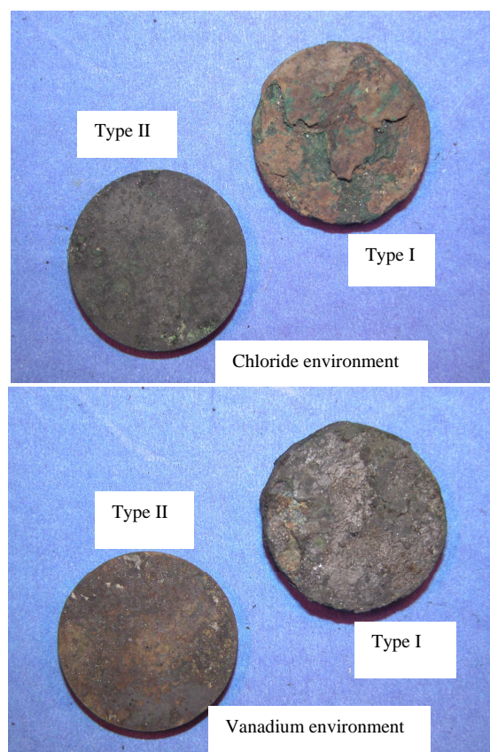
Figure 1. As hot corroded superalloy GTM-SU-263 in chloride and vanadium containing environments under type I and type II conditions.
