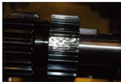
Figure 4. Test gear with a missing tooth.
