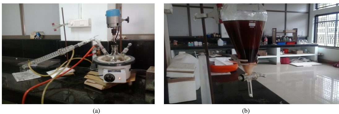
Figure 1. (a) Bench scale set up for biodiesel preparation; (b) product obtained after transesterification.
