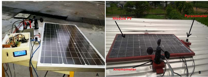
Figure 1. Acquisition station during the test (A) and after deployment (B) PV module, irradiation sensor, wind speed—UIT of Douala.
