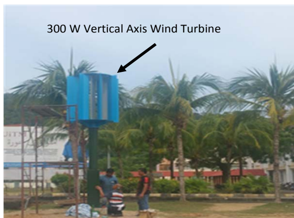
Figure 6. The 300 W vertical axis wind turbine generator.
